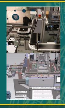
Manufacturing Execution System (MES) MES4 is a didactic structured Manufacturing Execution System (MES), which is designed for Industry 4.0 learning platforms. Special importance is placed on the topics of production control and management. The MES4 can directly communicate with the PLC via open communication interfaces. The individual controllers communicate with the MES4 via TCP/IP.
